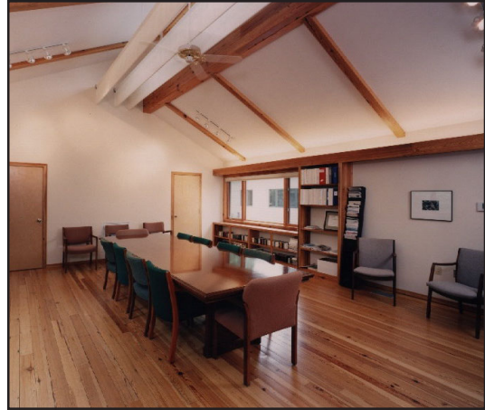
Conference room with South-facing clerestories for daylighting. Interior daylighting with supplemental energy efficient lighting reduces long-term operating costs and improves indoor environmental quality.
